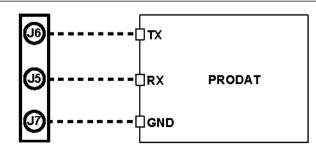
NOTE: PRODAT connected involves an output current error. Disconnect it to obtain a correct measure on output.
