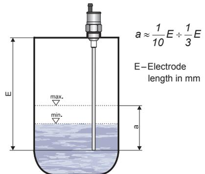
Fig. 11: Two state regulation by hysteresis setting
