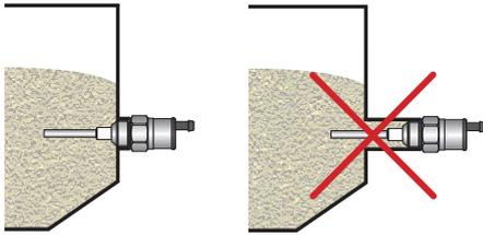
Fig. 2: Long fitting tubes in side wall mounting
