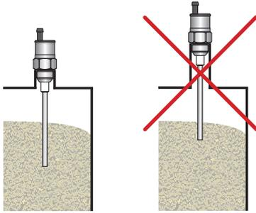
Fig. 12: Long fitting tubes in vertical mounting
