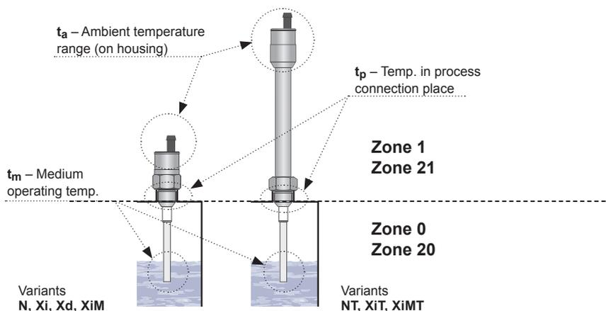
Fig. 15: Places for measurement of temperature and explosive areas
