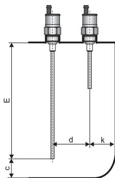
In the case of **vertical mounting** it is recommended to keep the mentioned distances applied to the length of the electrode (the longer one).
