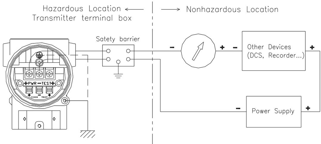
[Figure 4-3 Connection between Transmitter and Power Supply]
