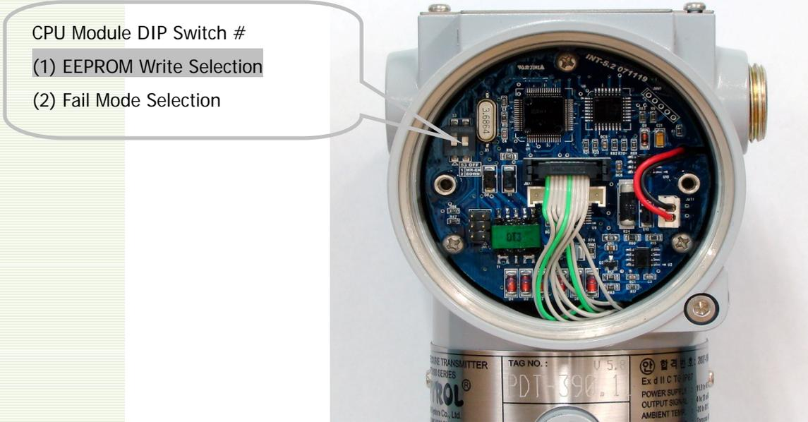
Figure 3-3. CPU Module EEPROM-Write Selection Jumper Switch location
