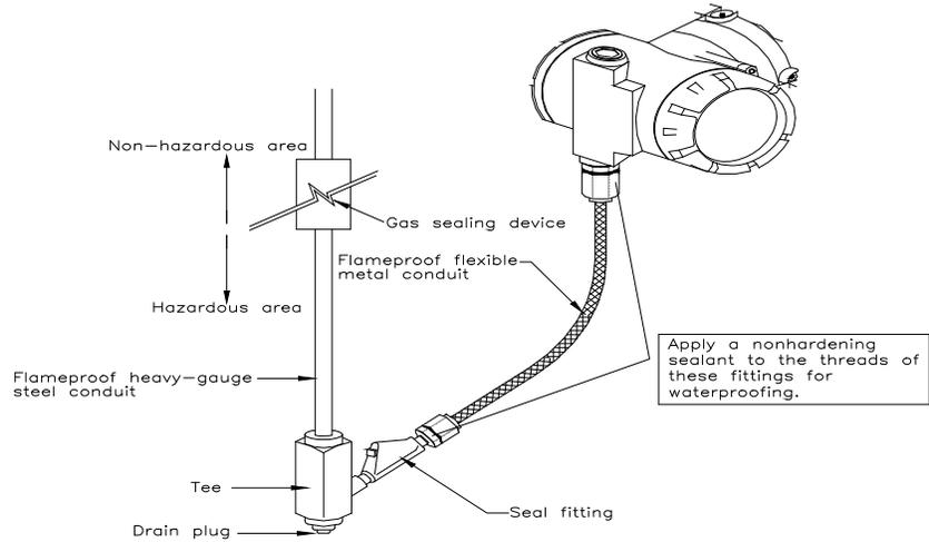
After wiring, impregnate the fitting with a compound to seal tubing.
