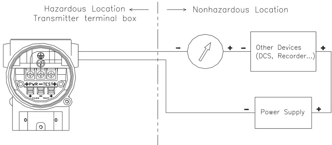
[Figure 4-3 Connection between Transmitter and Power Supply]
