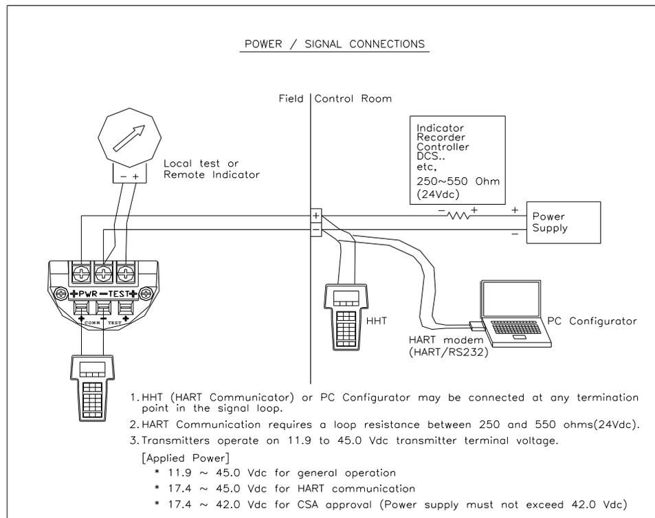
[Figure 3-5 Connection the transmitter to HHT]
