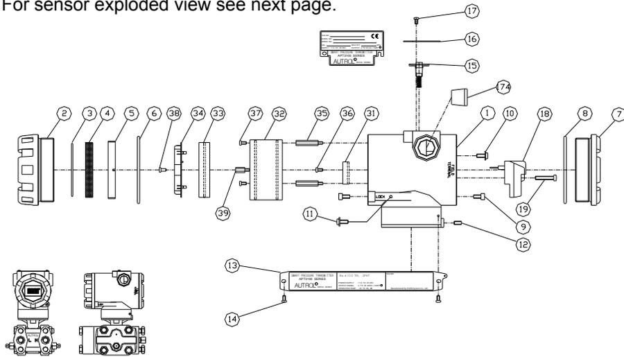
Figure 1-1. Model APT3100 Transmitter Exposed View (Housing)
