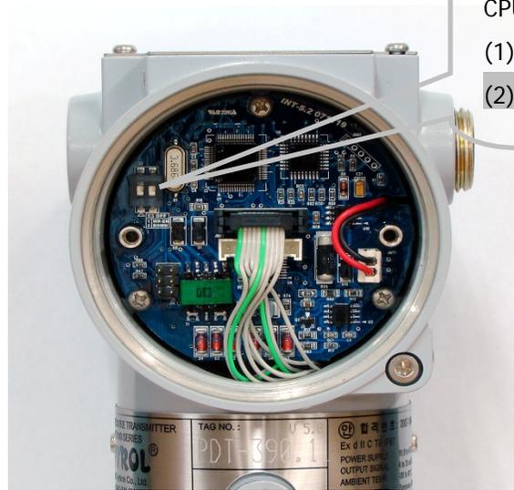
Figure 3-2. Fail Mode Selection DIP Switch location on CPU Board
